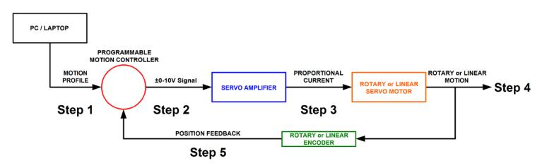
**Step 1.** A program or motion profile will be written on a PC or laptop and downloaded to the motion controller. This program will contain parameters such as speed, acceleration, deceleration, PIDs, desired position, etc...
